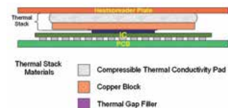
Figure 4: Construction detail of a thermal stack
